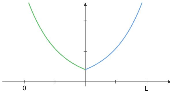
low-level injection prevails because  $\delta p = \gamma N_D \ll N_D$  since  $\gamma = 10^{-3}$ .
